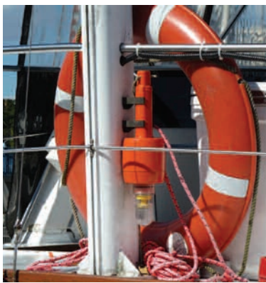
Keep a life ring and lighted buoy near the stern
