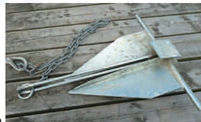
Danforth anchor with chain and shackle
